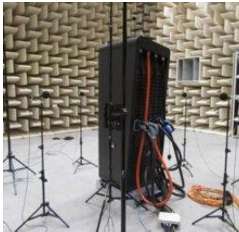
Figure 6: Acoustic measurement of an EVSE (Graphic courtesy of alpitronic GmbH).
