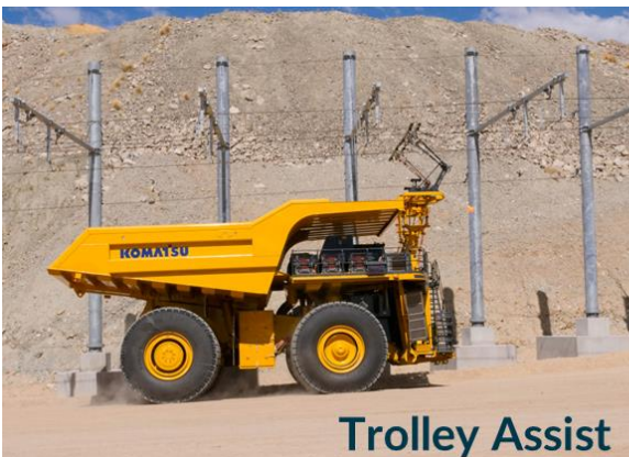
Figure 2.2 Dynamic charging technologies considered by this paper. Trolley assist systems (image courtesy of Komatsu) and side rail mounted system (image courtesy of BluVein).
