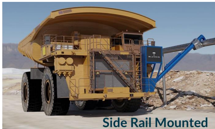
Figure 2.2 Dynamic charging technologies considered by this paper. Trolley assist systems (image courtesy of Komatsu) and side rail mounted system (image courtesy of BluVein).
