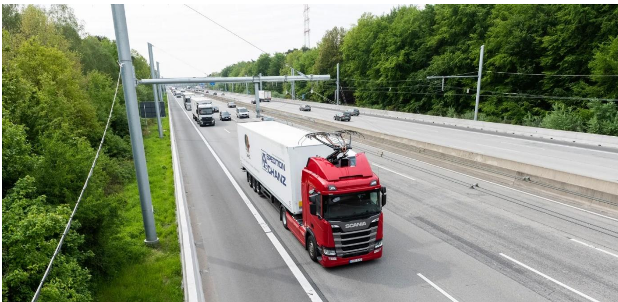
Figure 3.4 One of the Scania R450 hybrid trucks using the ELISA test track in Germany (image courtesy of Siemens Mobility).
